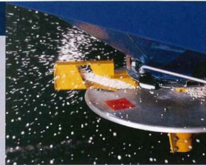
The discs rotate towards each other in the field (left) to provide the greatest accuracy of application. On the headland, the rotation of the discs is reversed (right), with the rear of the vanes creating a sharp headland cut-off.
